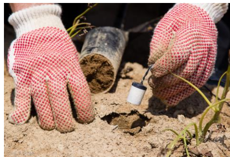
Fig.3 A gypsum block (“Soil-Moisture Sensor”).
